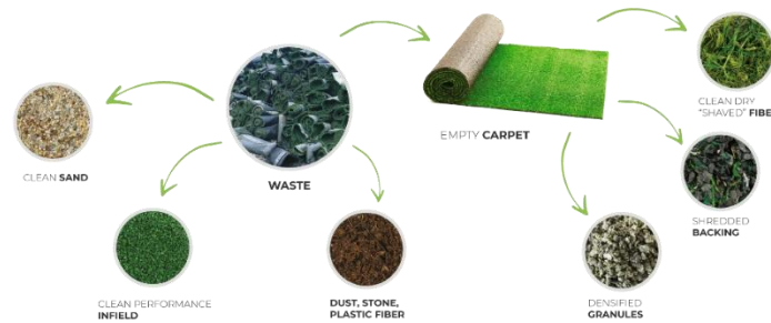
Figure 19: 100%TurfRecyclers' "from waste to resource" process
